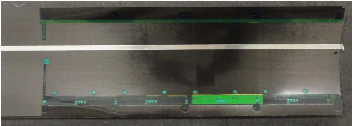
Figure 17: US bus tape co-cured with carbon fibre
